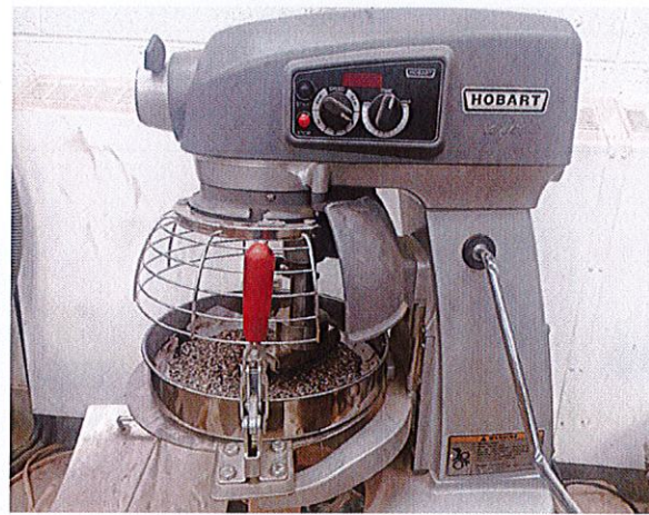
Fig. 4. Sweep test apparatus set-up.
